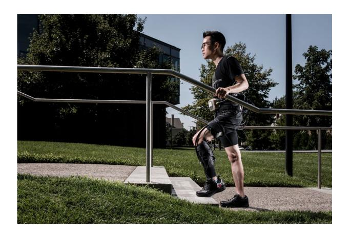
The soft robotic exosuit (shown here from the side) was worn by stroke patients on the hemiparetic side of their bodies. By assisting during the stance and swing phases of their gait cycles, it enabled them to walk faster and farther on a 30-meter walkway. Credit: Rolex Awards/Fred Merz
