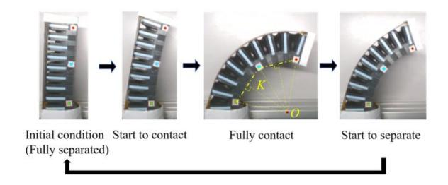
A working cycle of the soft robotic finger created by the researchers. Credit: Zhu et al.
