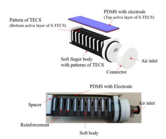
The reinforced soft finger with an embedded single-electrode triboelectric curvature sensor. Credit: Zhu et al.
