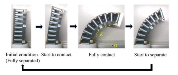
A working cycle of the soft robotic finger created by the researchers. Credit: Zhu et al.
