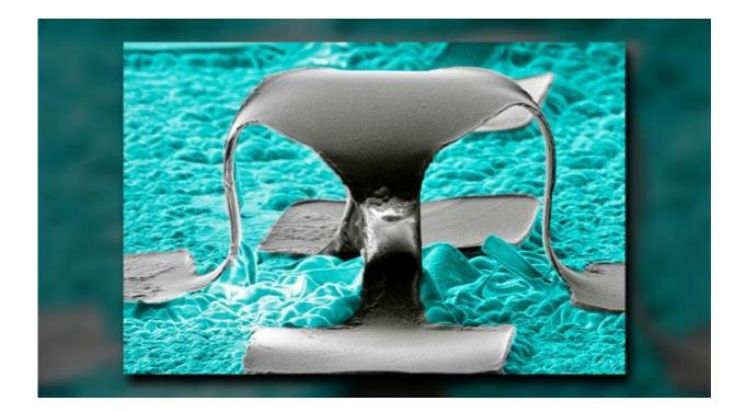
Electron micrograph of the tiny, table-shaped pressure sensor used in the study. Credit: Texas A&M University College of Engineering
