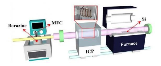
Remote ICP-CVD system with borazine mass flow controller (MFC) for precise control of borazine flow. The a-BN films were grown on Si substrates at 400 °C. Credit: UNIST, SAIT, University of Cambridge, Catalan Institute of Nanoscience and Nanotechnology
