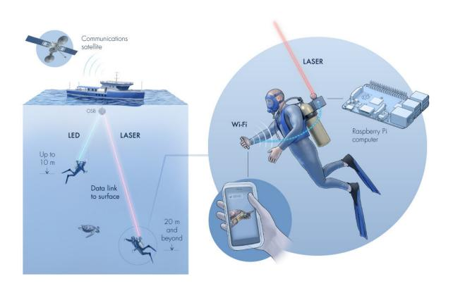
Aqua-Fi would use radio waves to send data from a diver's smart phone to a "gateway" device attached to their gear, which would send the data via a light beam to a computer at the surface that is connected to the internet via satellite. Credit: KAUST; Xavier Pita
