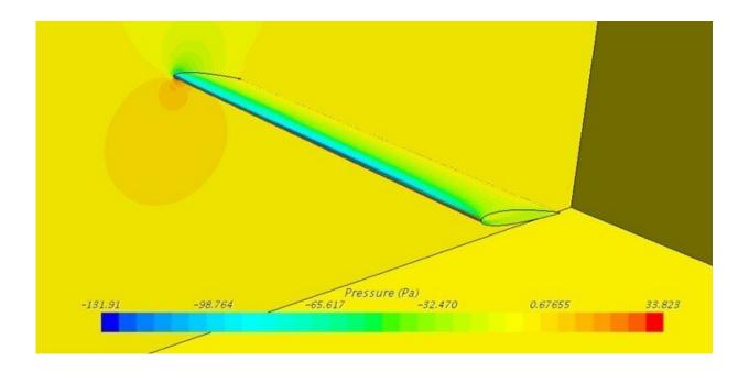
Researchers analyze a simulated air pressure field over a deformed wing inside a wind tunnel. Credit: U.S. Army
