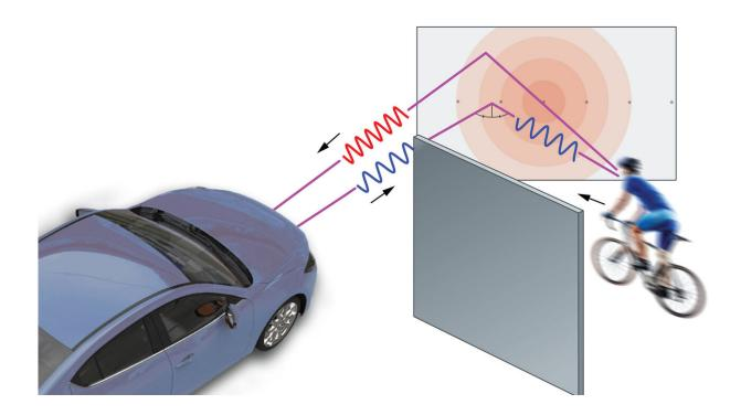
Researchers combined artificial intelligence and radar used to track speeders to develop a system that will allow vehicles to spot hazards hidden around corners. Image courtesy of the researchers.
