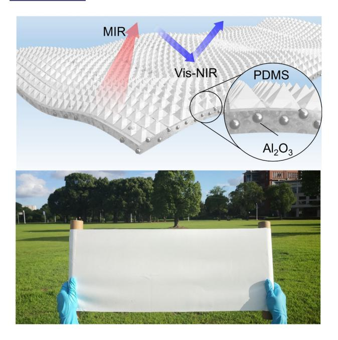
Structure of the bioinspired hybrid film with ceramic particles embedded in the micro-pyramid polymer matrix. Credit: Haiwen Zhang.
