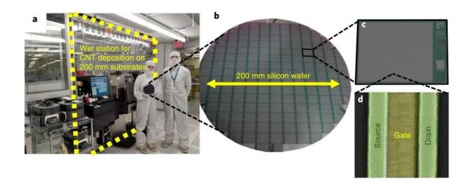
Integration of CNFETs within a commercial silicon foundry. Credit: *Nature Electronics* (2020). DOI: 10.1038/s41928-020-0419-7
