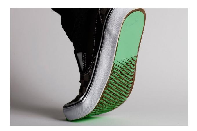
MIT researchers drew on kirigami, a variation of origami that involves cutting paper as well as folding it, to create a friction-boosting material that could be used to coat the bottom of your shoes, giving them a stronger grip on ice and other slippery surfaces. Credit: Diemut Strebe
