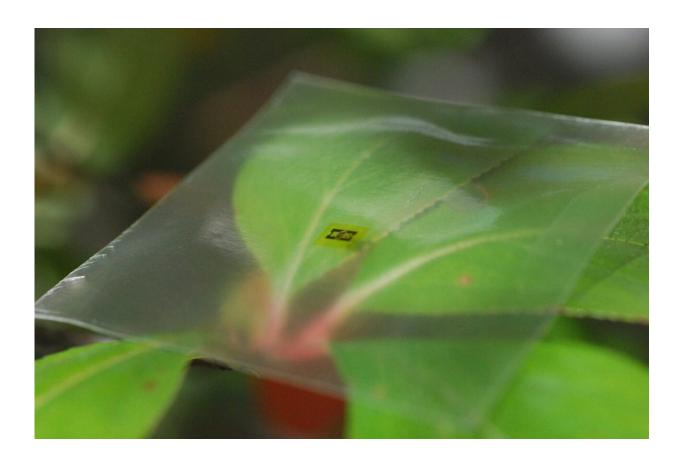
UW-Madison engineers and collaborators have constructed a functional microwave amplifier circuit — a common piece of electronics used in wireless communications — on a flexible substrate made of wood fiber. Credit: Huilong Zhang
