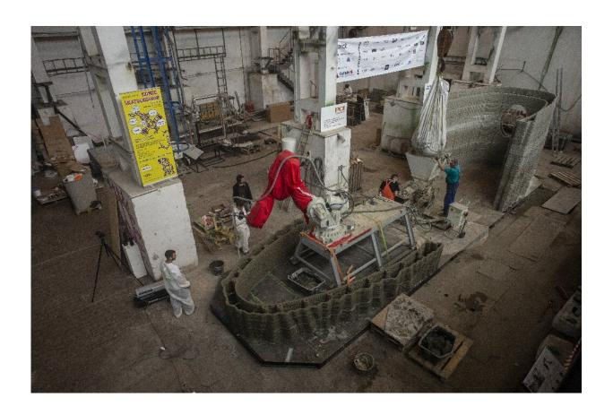
Workers check over the 3D construction, which is being printed from special concrete and is due to float down the river Vltava in August
