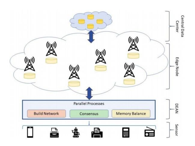
A figure showing a possible four-tier edge computing architecture integrating the protocol devised by the researchers. Credit: Al-Mamun & Zhao.
