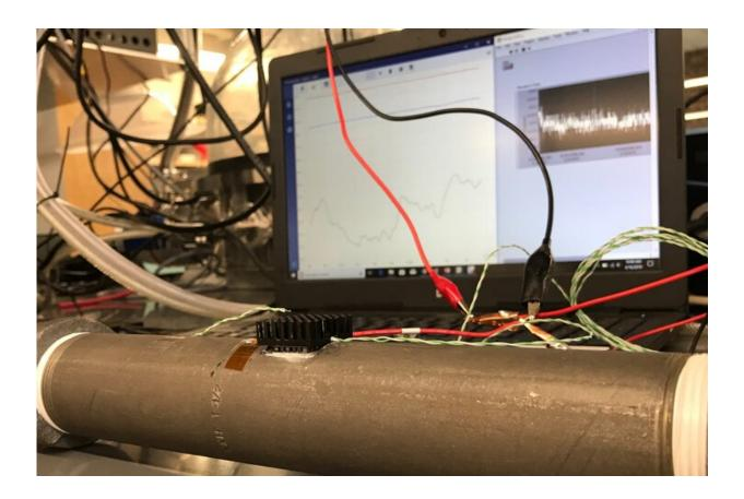
Scientists test the performance of a thermoelectric device. The devices can efficiently convert wasted heat from sources like hot water pipes into usable electricity, scientists said. Credit: Penn State
