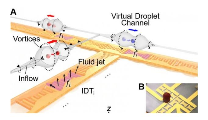
Droplets of different sizes sit on grids of transducers that vibrate to create tunnels in a thin layer of oil, which can transport the droplets in multiple directions. Credit: Duke University
