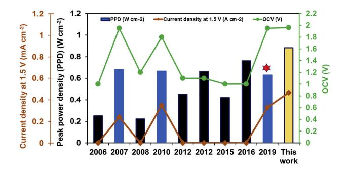
The figure summarizes open circuit voltages of the representative DBFC performance in green and current density at 1.5 V in orange. DBFCs with peak power density at high voltage (>1 V) are represented by blue columns and those with peak power density at low voltage (
