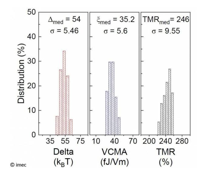
Figure 2: Figures of merit for the VCMA MRAM device. The graph shows distributions of the fundamental parameters for the baseline devices, with  $\Delta$  = 54, VCMA coefficient = 35.2fJ/Vm and TMR = 246% in median. Credit: IMEC
