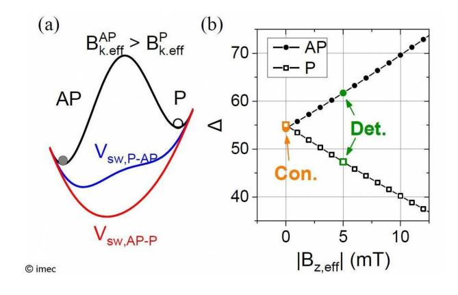
Figure 1: (a) Energy diagram with Bz,eff for the proposed deterministic write, where the AP state is more stable than the P state. (b) Retention ( $\Delta$ ) as a function of Bz,eff. Credit: IMEC
