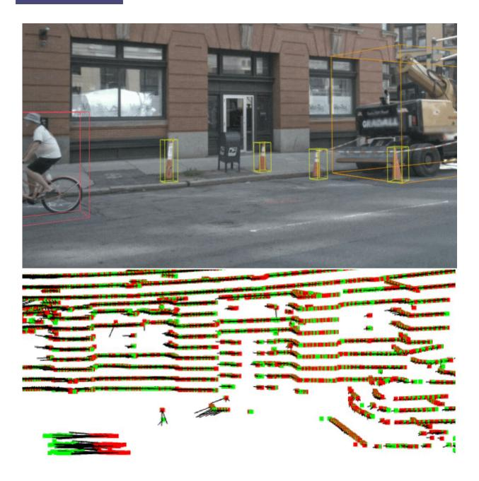
A technique called scene flow can be used to predict the future position of a cyclist by comparing the current lidar point cloud of a street scene, in green, with the point cloud from the previous time step in the sequence, shown in red. Carnegie Mellon University researchers have developed a method that increases the amount of data available for training such systems. Credit: Carnegie Mellon
