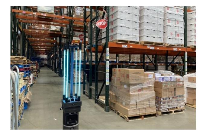
The approach uses a custom UV-C light fixture designed at CSAIL that is integrated with Ava Robotics' mobile robot base. Credit: Alyssa Pierson/CSAIL
