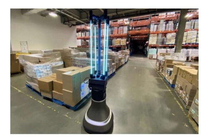
In tests, the CSAIL team's robot could disinfect a 4,000-square-foot space in the food bank's warehouse in just half an hour. Credit: Alyssa Pierson/CSAIL
