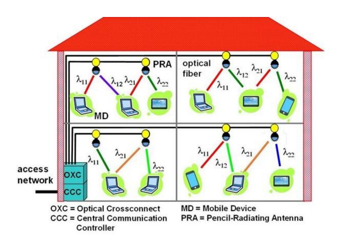
An example of an indoor optical wireless communication system using narrow infrared beams. Credit: Eindhoven University of Technology
