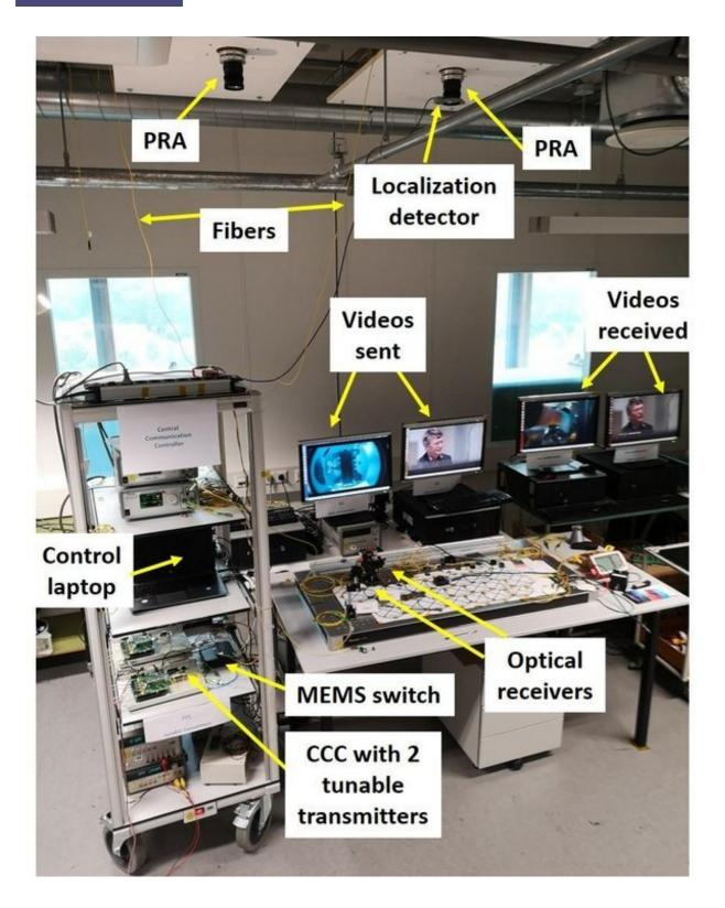
Demonstration of an infrared wireless communication system in Ton Koonen's lab.
