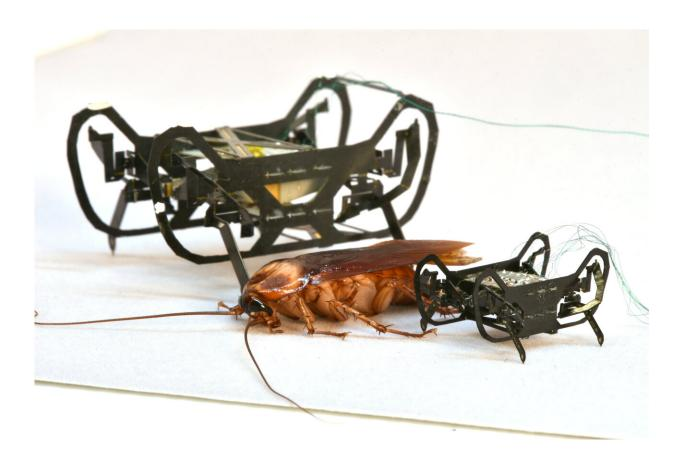
The newly designed HAMR-Jr alongside its predecessor, HAMR-VI. HAMR-Jr is only slightly bigger in length and width than a penny, making it one of the smallest yet highly capable, high-speed insect-scale robots. Credit: Kaushik Jayaram/Harvard SEAS
