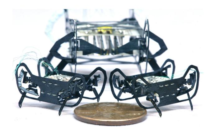
The newly designed HAMR-Jr alongside its predecessor, HAMR-VI. HAMR-Jr is only slightly bigger in length and width than a penny, making it one of the smallest yet highly capable, high-speed insect-scale robots. Credit: Kaushik Jayaram/Harvard SEAS
