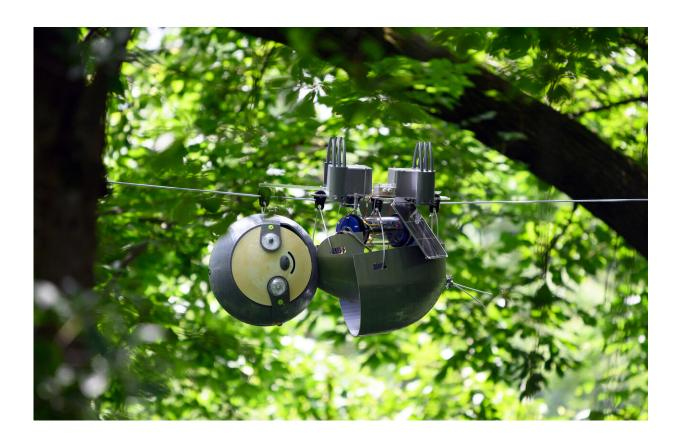
SlothBot is a slow-moving and energy-efficient robot that can linger in the trees to monitor animals, plants, and the environment below. It has been installed for testing in the Atlanta Botanical Garden. Credit: Rob Felt, Georgia Tech
