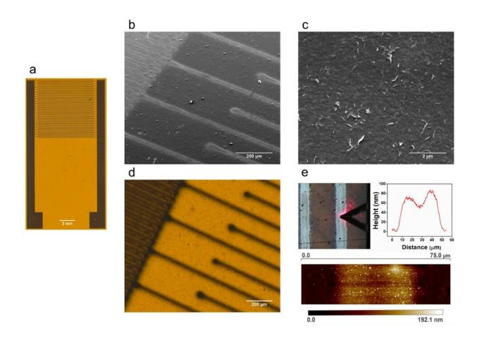
Researchers are using aerosol-jet-printing technology to create these graphene biosensors that can detect histamine, an allergen and indicator of spoiled fish and meat. Credit: Jonathan Claussen/Iowa State University
