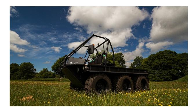
A hybrid electrical powered version of the All-Terrain Mobility Platform (the ATMP) Credit: Supacat and SC Innovation as part of SC Group.
