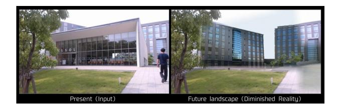
Proposed "diminished reality" (DR) system. Left: Input image captured by a web camera showing the current situation. Right: DR output image of the future landscape. A moving object (pedestrian) has been virtually removed in real-time along with the immobile building.? Credit: Osaka University
