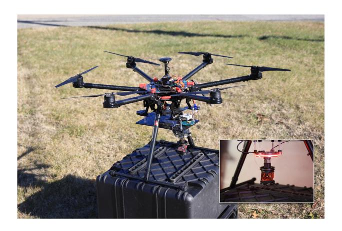
A UAS outfitted with both a marker strobe (inset) and a traditional survey prism used to evaluate the accuracy of the motion-capture system. Credit: U.S. Army
