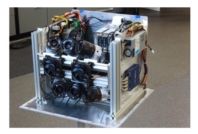
Each of the 16 tracking pod includes six cameras with overlapping fields of view. Credit: U.S. Army
