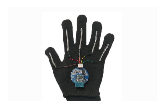
The system includes gloves with thin, stretchable sensors that run the length of each of the five fingers. Credit: Jun Chen Lab/UCLA
