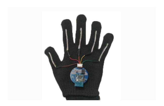
The system includes gloves with thin, stretchable sensors that run the length of each of the five fingers. Credit: Jun Chen Lab/UCLA
