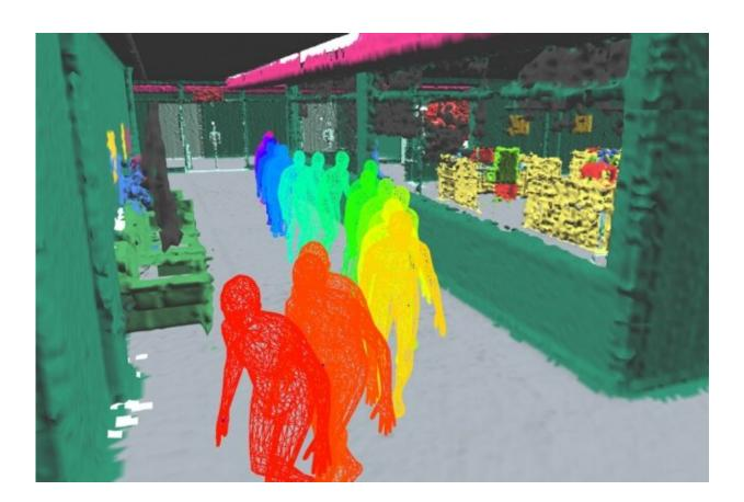
MIT researchers have developed a representation of spatial perception for robots that is modeled after the way humans perceive and navigate the world. The key component of the team's new model is Kimera, an open-source library that the team previously developed to simultaneously construct a 3D geometric model of an environment. Kimera builds a dense 3D semantic mesh of an environment and can track humans in the environment. The figure shows a multi-frame action
