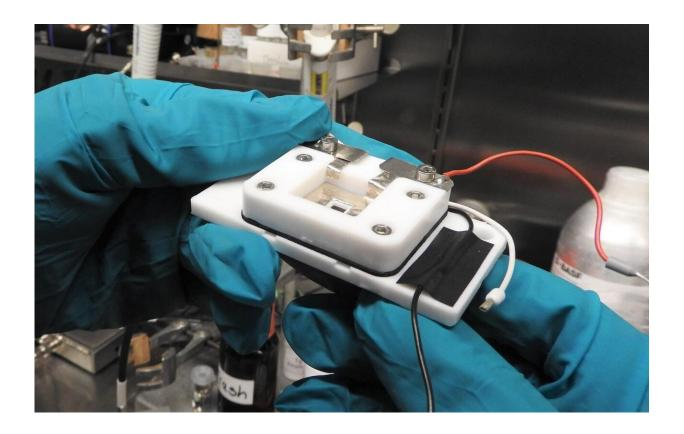
In a measuring cell developed in-house, the Oldenburg team examined lithium electrodes using electrochemical scanning microscopy. Credit: Bastian Krueger
