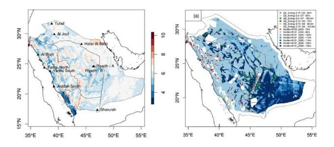
Four-year average wind speed (left) and optimal wind turbine technology (right) for Saudi Arabia. Credit: Reproduced under a Creative Commons license from reference one, 2020 Genton et al.
