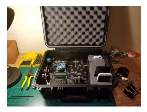
Inside the Beamlink case: a cellular base station, test mobile phones and a portable EKG device. Credit: Arpad Kovesdy
