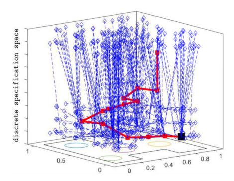
As a control algorithm moves robots through a space, each state the robots can be in is represented by a spot on the 3D graph. As the algorithm explores new options, it finds failures and potential next moves. This graph represents all of the wrong moves explored (blue) and the one route that is correct (red). Credit: Michael Zavlanos, Duke
