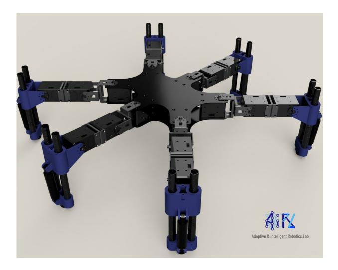
The hexapod robot on which the researchers tested their algorithm. Credit: Adaptive & Intelligent Robotics Lab, Imperial College London.
