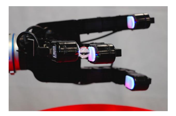
DIGIT sensors mounted on an Allegro multi-fingered hand. Credit: Lambeta et al.
