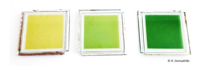
The solar cells developed by the researchers in their different color conditions. Credit: Demadrille et al.
