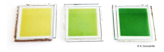
The solar cells developed by the researchers in their different color conditions. Credit: Demadrille et al.
