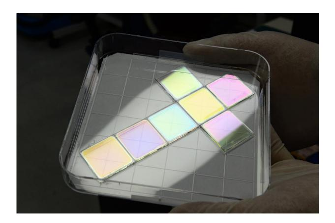
The eco-friendly color CIGS thin film solar cells developed by ETRI researchers. Credit: Electronics and Telecommunications Research Institute (ETRI)
