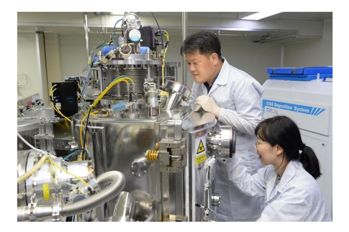
ETRI researchers are monitoring the thin film solar cell process with CIGS deposition equipment. Credit: Electronics and Telecommunications Research Institute (ETRI)
