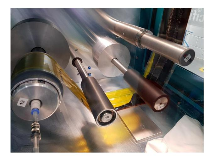
Thin flexible films with printed solar cells are a key step towards cheaper and more efficient solar energy - Swansea University researchers have demonstrated record efficiency levels for perovskite solar cells Credit: SPECIFIC/Swansea University
