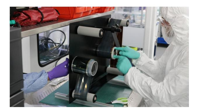
Two-step roll to roll coating of perovskite thin films at Swansea University, where researchers from the SPECIFIC project have achieved record efficiency levels for printed solar cells. Credit: SPECIFIC/Swansea University
