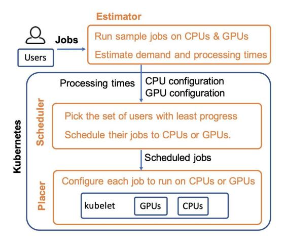
The AlloX system has three main components: an estimator, a scheduler, and a placer, which together determine which hardware best serves a job and then how to most fairly fit it into what's currently available. Credit: University of Michigan
