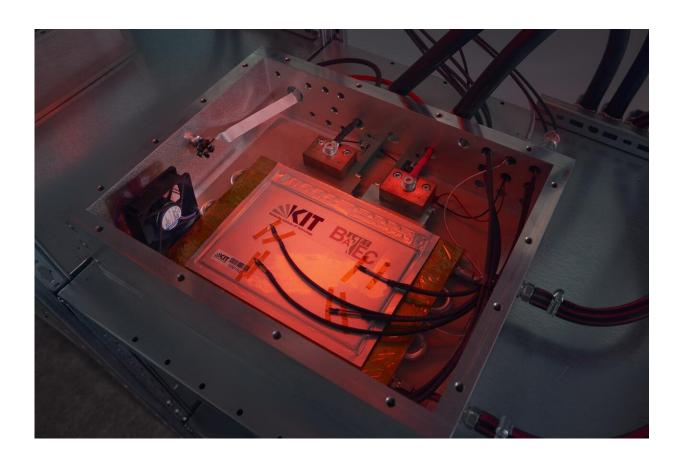
KIT developed a temperature-controlled safety housing that is equipped with a sensing system for testing lithium-ion cells under critical conditions. (Photo: Amadeus Bramsiepe, KIT) Credit: Amadeus Bramsiepe, KIT
