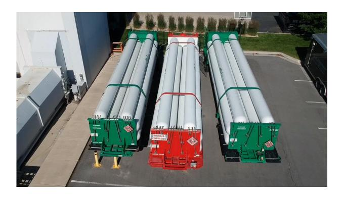
Microsoft used hydrogen stored in these tanks on trailers parked outside a lab near Salt Lake City, Utah, to fuel hydrogen fuel cells that powered a row of
