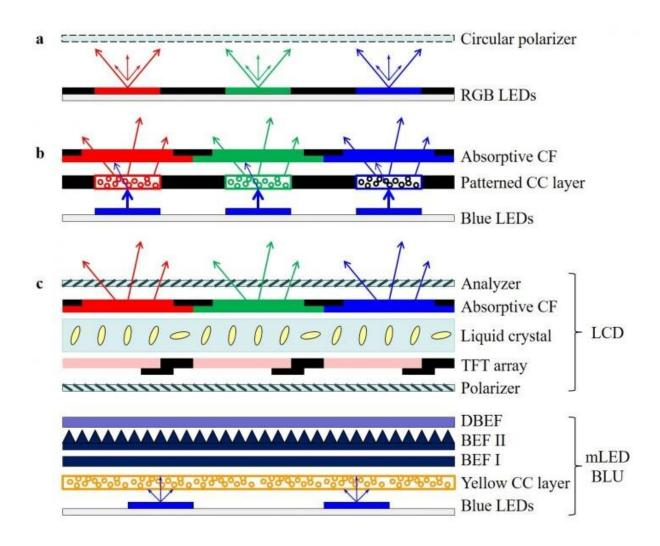
a. RGB-chip mLED/ $\mu$ LED/OLED emissive displays. b. color conversion mLED/ $\mu$ LED/OLED emissive displays. c. mini-LED backlit LCDs. CF: color filter; CC: color conversion; TFT: thin-film transistor; DBEF: dual brightness enhancement film; BEF: brightness enhancement film; BLU: backlight unit.
