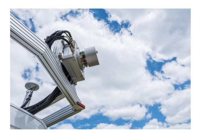
3D laser scanner contained in a housing and mounted on the roof of a vehicle. Credit: Fraunhofer IPM
