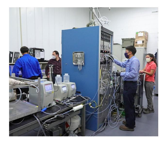
The Particle Science and Technology Laboratory is ISO/IEC 17025-accredited by the American Association for Laboratory Accreditation to calibrate devices that measure particles as small as 10 nanometers in diameter. Recent mask testing at SwRI revealed more than two-thirds of KN95 respirator samples submitted by health care and government clients did not meet U.S. standards for filtration efficiency. Credit: Larry Walther, SwRI
