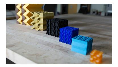
Several metamaterial prototypes at different scales, which were miniaturized at the micron scale using two-photon direct laser writing. Credit: Allison L. Carter, Georgia Tech
