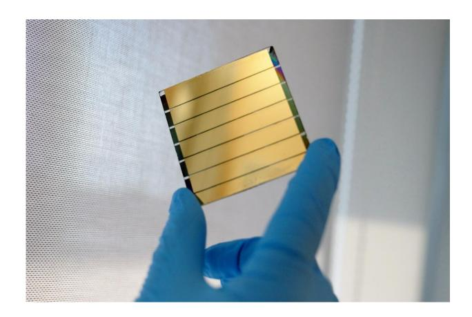
Perovskites can be used to create light-weight flexible and semi-transparent solar cells ideal for applications in buildings and a variety of urban spaces. Credit: NTU Singapore
