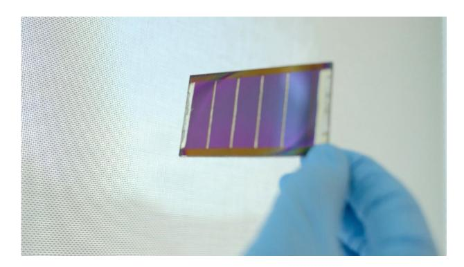
The colored semi-transparent version of a perovskite solar mini module achieved similar measures of power conversion efficiency across a whole range of different colors. Credit: NTU Singapore
