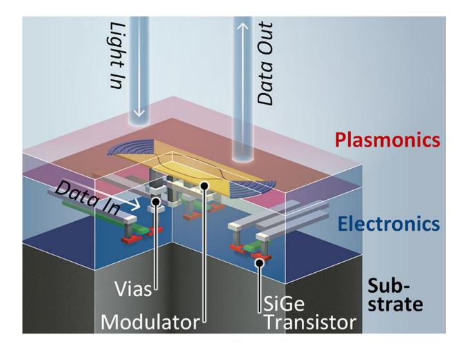
Thanks to the combination of electronics and plasmonics on a single chip, light signals can be amplified and data can be transmitted faster. Credit: IEF/Springer Nature Ltd.
