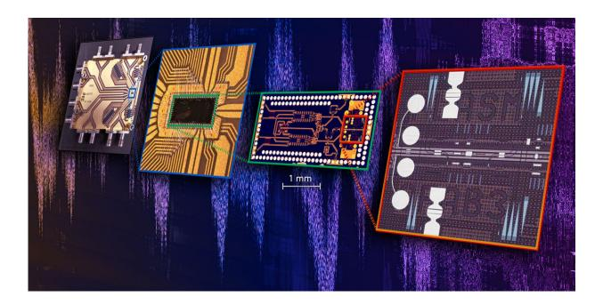
The new, highly compact chip brings together the fastest electronic and lightbased elements in a single component for the first time. Credit: ETH Zurich/Nature Electronics
