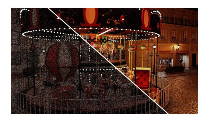
ReSTIR dramatically increases the quality of rendering on a computer's graphics card by reusing rays that were traced in neighboring pixels and in prior frames. This photo compares the ReSTIR (r) rendering process with an older technique (l). Credit: Amazon, Turbosquid, Kate Anderson.
