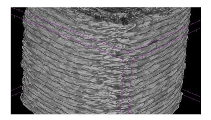
A three-dimensional view of a reconstructed CT scan model of a 3D printed composite part showing overall dimensions and geometry. Credit: NYU Tandon School of Engineering
