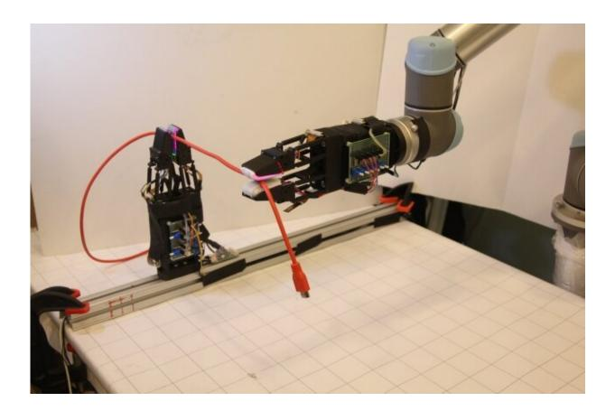
The system uses a pair of soft robotic grippers with high-resolution tactile sensors to successfully manipulate freely moving cables. Credit: MIT CSAIL
