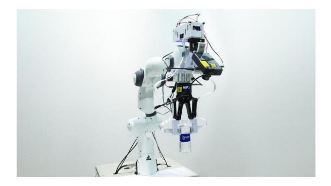
This novel robotic system developed by NUS researchers comprises an artificial brain system that mimics biological neural networks, which can be run on a power-efficient neuromorphic processor such as Intel's Loihi chip, and is integrated with artificial skin and vision sensors. Credit: National University of Singapore
